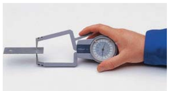
Testing the residual material thickness ST
