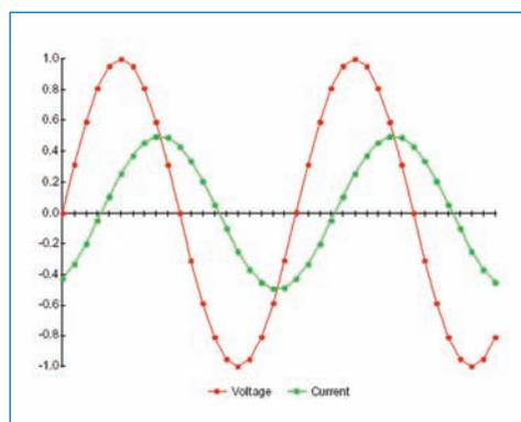
The relationship between the voltage and current can also be shown using vectors and this approach allows easy calculation of the rating of power factor correction equipment.
