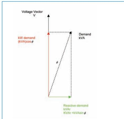
By installing a capacitor bank to draw capacitive (leading) current, the inductive or lagging element of current can be reduced and the resultant total current (and kVA demand) can be reduced. See Figure 4.
