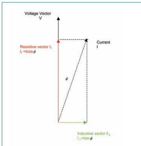
The cosine of the angle  $\phi$  between the current (I) and the voltage vector (V) is called the power factor.
