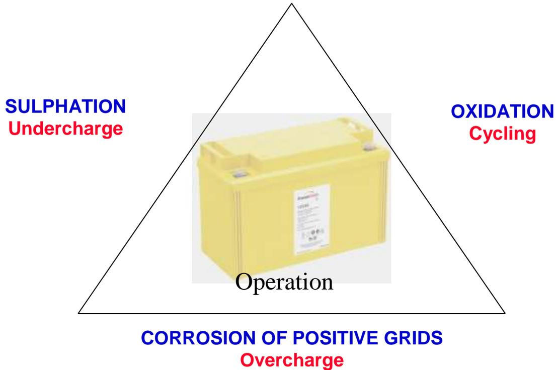
Another factor to be considered is the working temperature. An increase of 10 °C in the temperature, from 20 to 30 °C, will halve the life of the battery; a further increase of 10 °C will halve it again ( thus reducing its expected life to one quarter).
