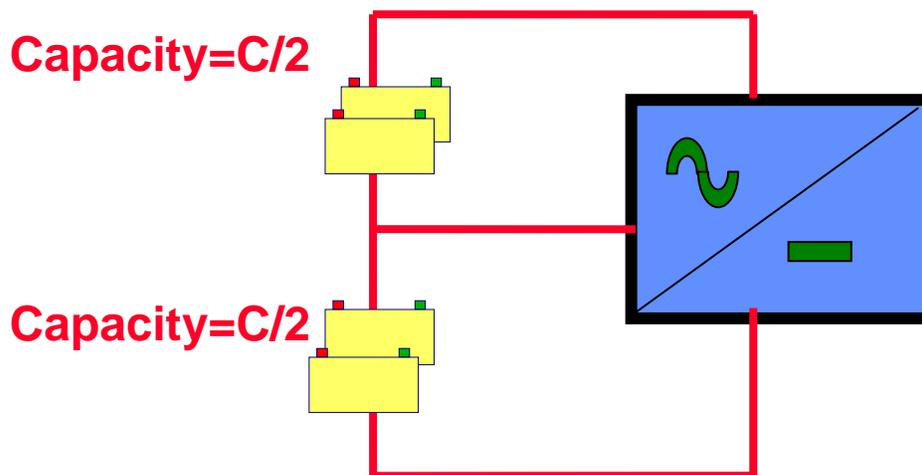
*Wiring diagram with redundant batteries*
