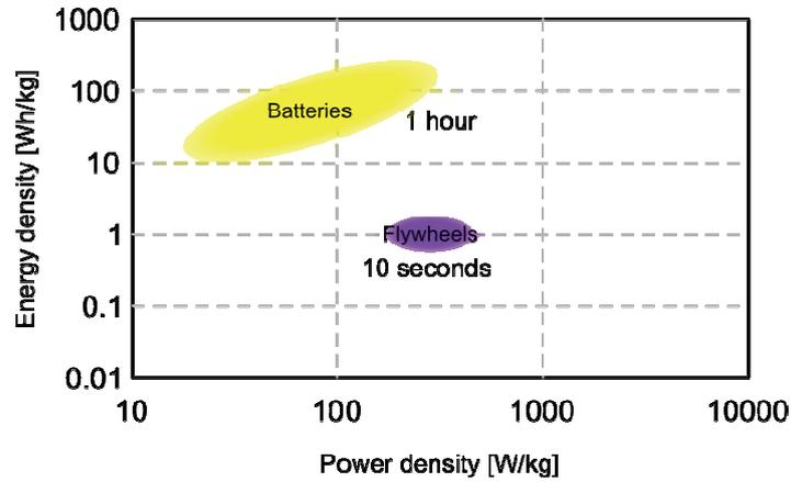
Last but not least, flywheels can be installed in place of batteries or even in parallel with them on the DC BUS. The advantage of a hybrid battery/flywheel energy storage system is that in the event of micro-interruptions the flywheel is able to supply the energy needed by the system, whereas the batteries are only required for outages lasting longer than 10 seconds, thereby extending the life of the accumulators.
