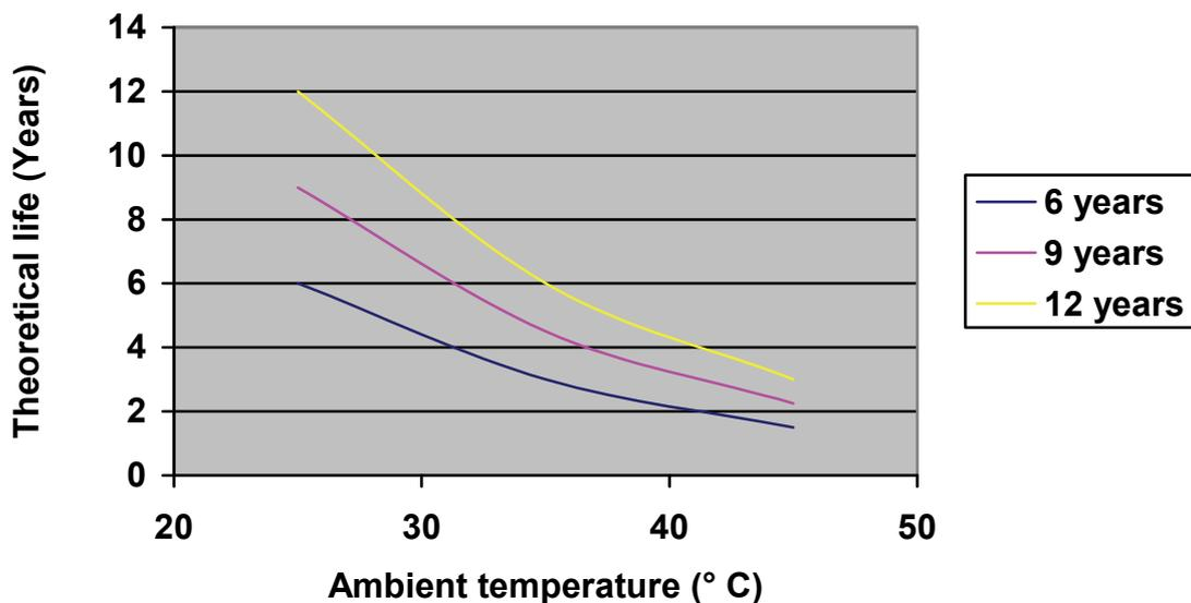
Furthermore batteries are extremely sensitive to the amount and type of usage: charge and discharge cycles, discharge depth and current, charging method, etc. Therefore it is advisable to choose a UPS system with, among other things, a very stable, temperature-dependent charging current, with control systems to identify damaged elements which would cause overload of healthy elements and rectifiers with a wide input tolerance range, so that batteries are used as little as possible.
