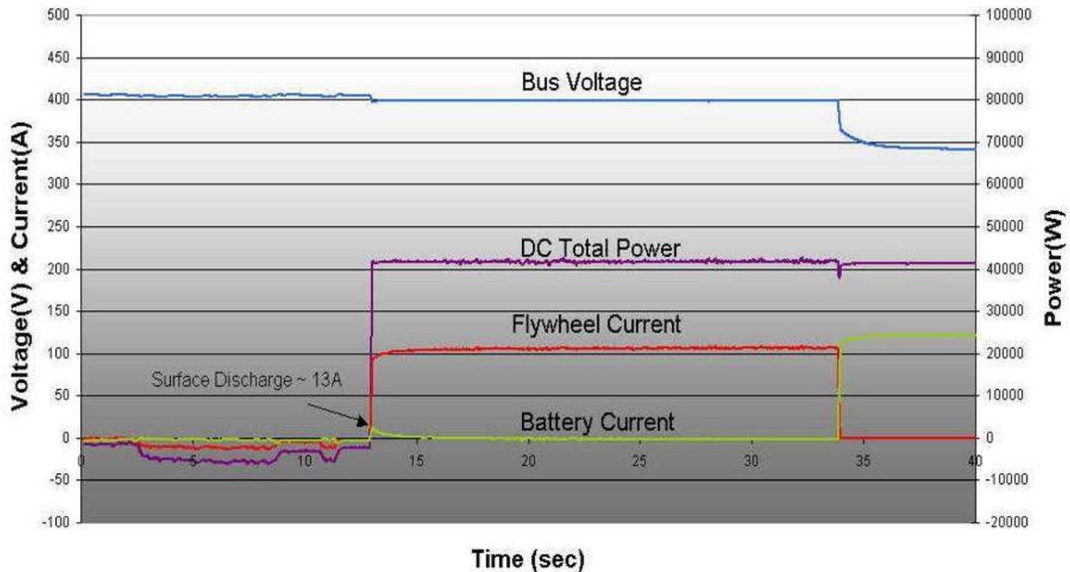
FIG. 5 - UPS INTEGRATION BATTERY IN PARALLEL
