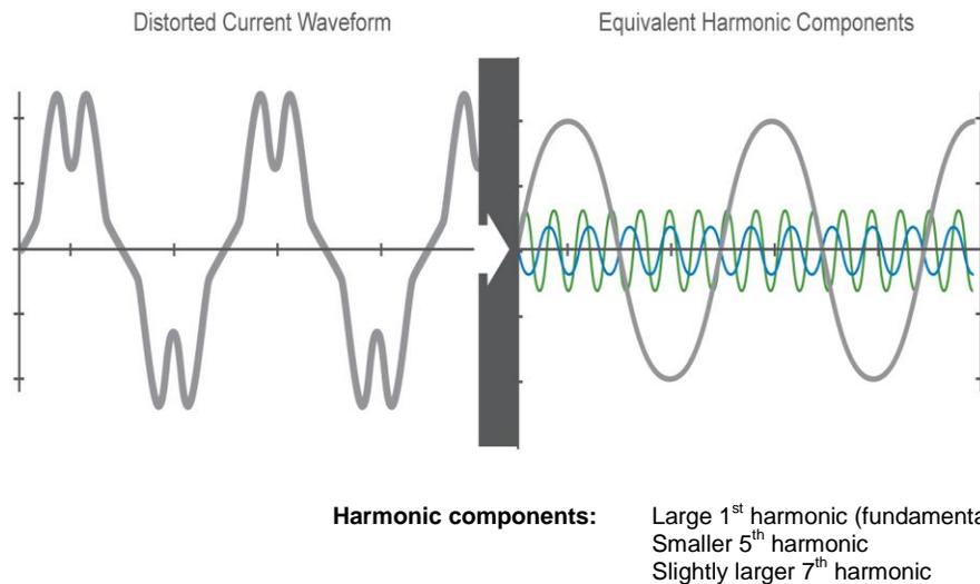
**Figure 2. Distorted waveform composed of fundamental, 5<sup>th</sup> and 7<sup>th</sup> harmonics**
