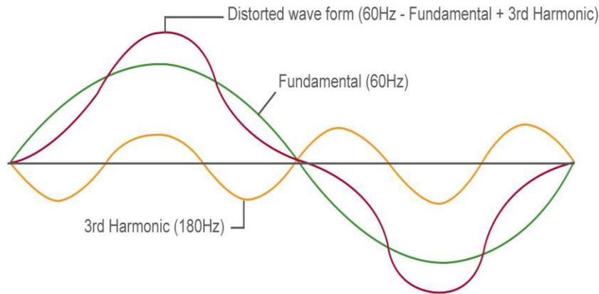
**Figure 1. Harmonic distortion of the electrical current waveform**
